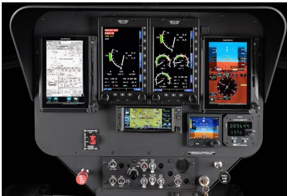
Glass Cockpit with Howell Instruments Engine Instruments Display, Garmin G500H TXi™ MFD/PFD, L3Harris ESI-500 and GTN™ 650H. (optional equipment also depicted)
